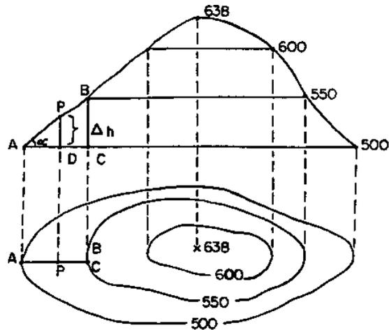
Altura do ponto P:  $H P = 500\text{m} + \overline{PD} (\Delta h)$
