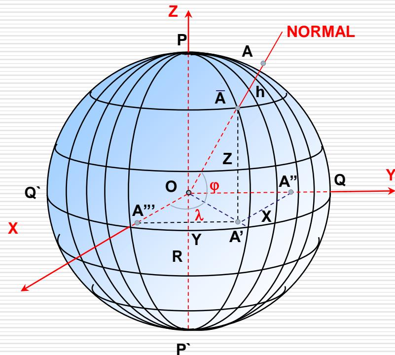
$$\begin{aligned}x &= (R+h) \cos \varphi \cos \lambda \\y &= (R+h) \cos \varphi \sin \lambda \\z &= (R+h) \sin \varphi\end{aligned}$$
